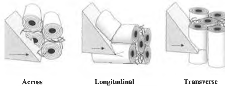
Figure 2.19: Illustration of the cutting modes relative to predominant osteon direction (Plaskos et al., 2003)
