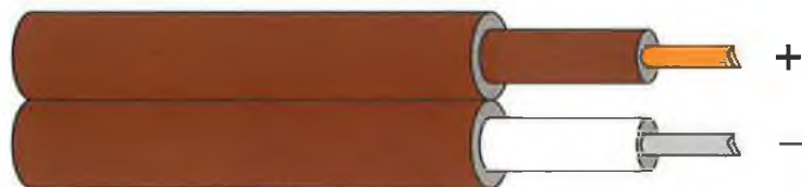
Figure 3.3: Illustration of thermocouple type T international color code
