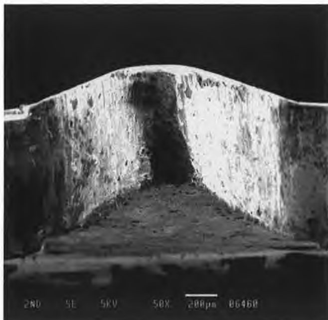
Figure 4.23: SEM image of cutting edge of the used blade
