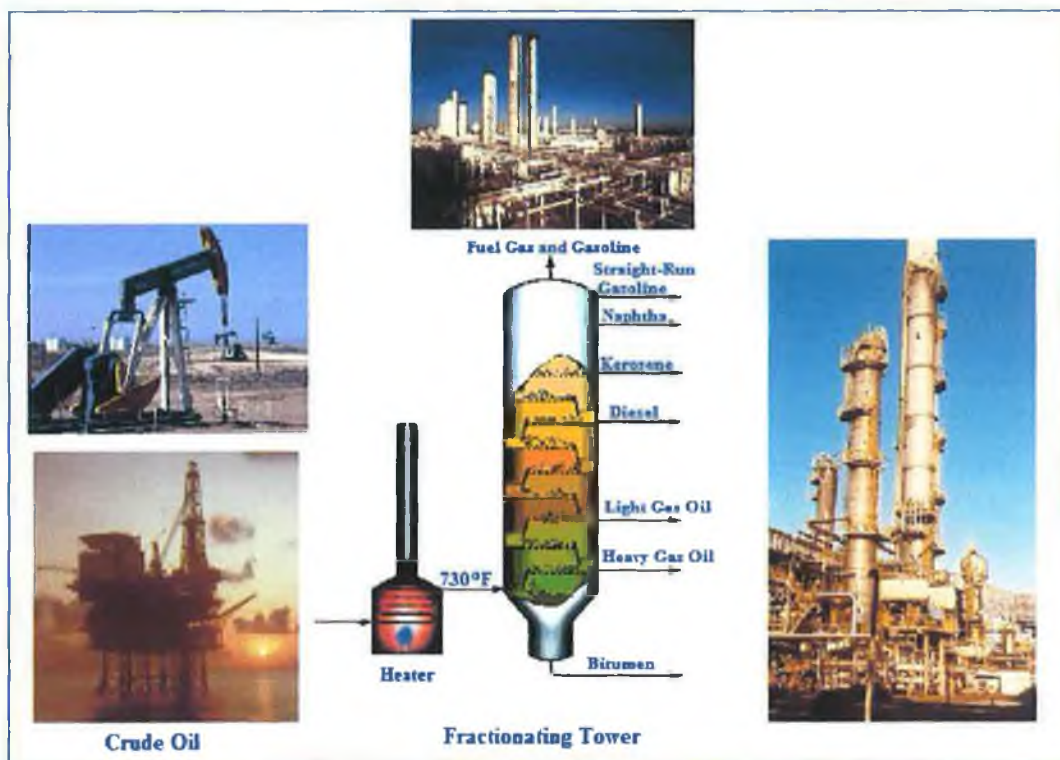
Figure 1.1 Crude Oil Distillation Process
