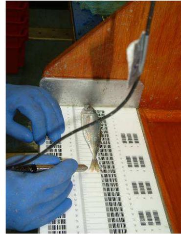
Figure 2. Electronic measuring board. Each 1cm length class corresponds to a barcode that is read with a light pen.
