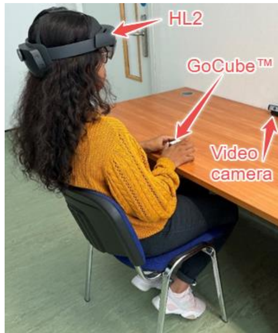
Fig. 5.2. Study 2 test set-up showing a participant wearing the HL2, holding the GoCube™ with the 1080p Logitech desk mounted camera.
