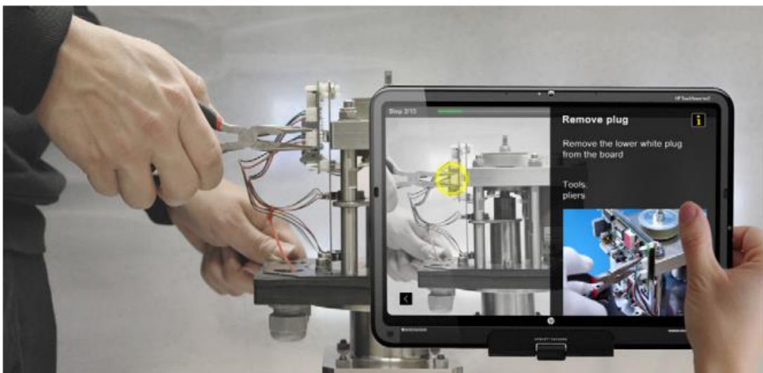
Fig. 2.4. An example of target object pattern recognition in the absence of fiducial markers [44].
