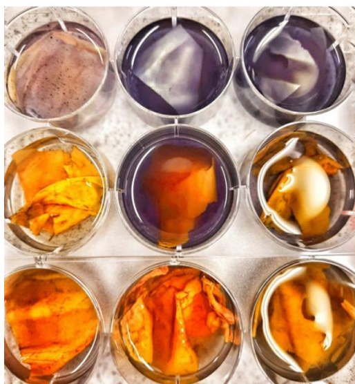
Figure 16. BC materials immersed in TSNP solution for overnight incubation. Bare BC films and Curcumin-BC films are included. Top row: Bare BC, middle row: BC-Cur2%, bottom row: BC-Cur10%.
