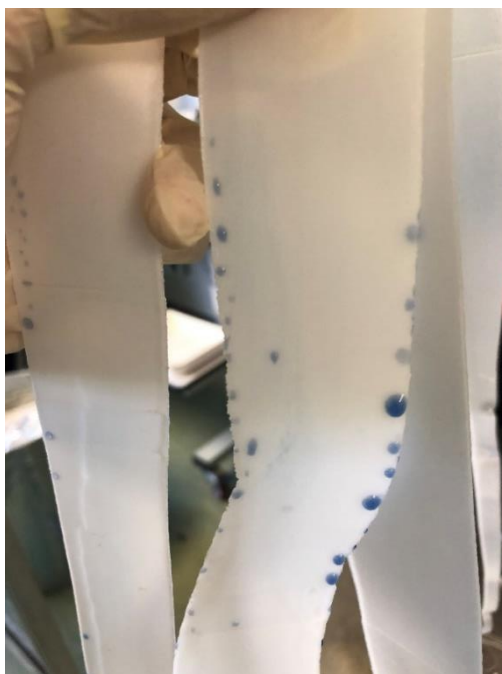
Figure 33. Post-extrusion addition of TSNP (in water solution). The blue spots show drops of TSNP solution which could not be absorbed by the polymer even in a melted state, due to its hydrophobicity.
