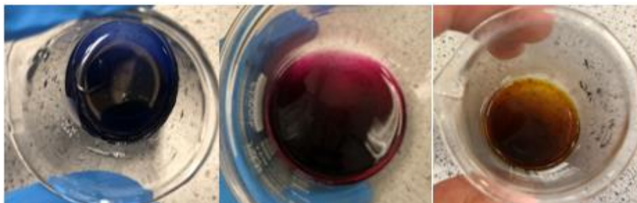
Figure 28. Colour of TSNP solution before and after evaporation process: Left) Initial colour of TSNP solution; Centre) Final colour of sample A; Right) Final colour of sample B.
