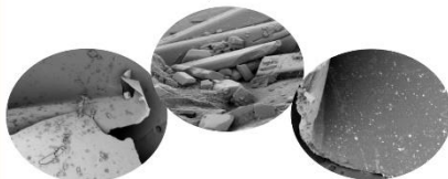
Figure 2. SEM micrographs of BC/Cur 100x (Left), BC/Cur 1.2kx (Center) and BC/TSNP 115x (Right).
