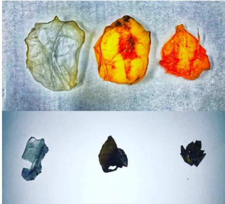
Figure 55. Top) BC produced in regular HS medium (Left), in 2% curcumin supplemented (Center) and in 10% curcumin supplemented (Right). (Bottom) Regular BC (Left), BC with 2% supplemented curcumin (Center) and BC with 10% supplemented curcumin (Right) after TSNP
