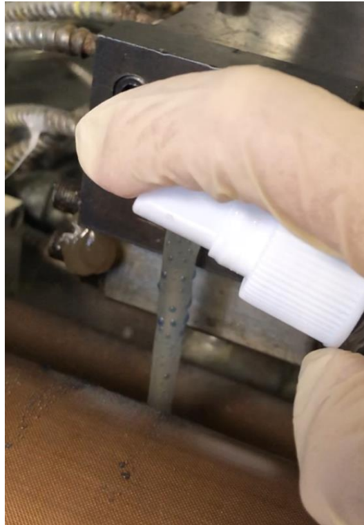
Figure 15. Spraying TSNP solution as the PCL exits the extrusion die and goes through the rolls.
