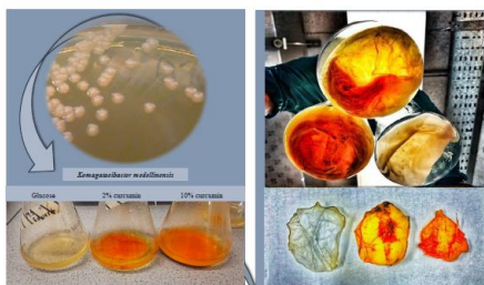
Figure 2. Wet (top) and dried (bottom) BC after cultivation in regular HS medium and medium supplemented with 2% and 10% of curcumin, respectively.
