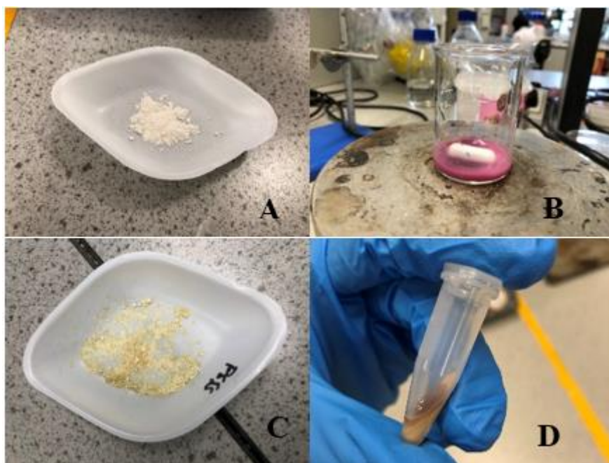
Figure 30. Mixed TSNP+HNT: A) Pure HNT Powder; B) TSNP+HNT solution; C) Dried and ground TSNP+HNT; D) Centrifuged TSNP+HNT.
