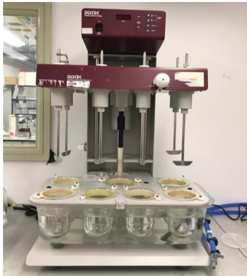
Figure 1. Dissolution tester to study the %drug release
