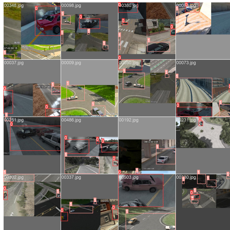
Figure 3. Customised (annotated) synthetic data used in training of YOLOv5 (bounding boxes drawn on event occurred: 0 (red color) and 1 (pink color) represents accident and non-accident, respectively).
