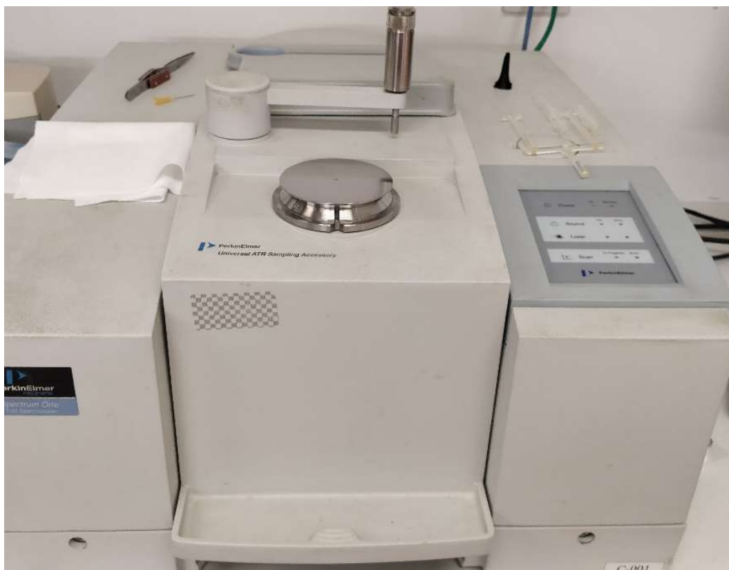
Figure 3-7 Perkin Elmer Spectrum One fitted with a universal ATR sampling accessory
