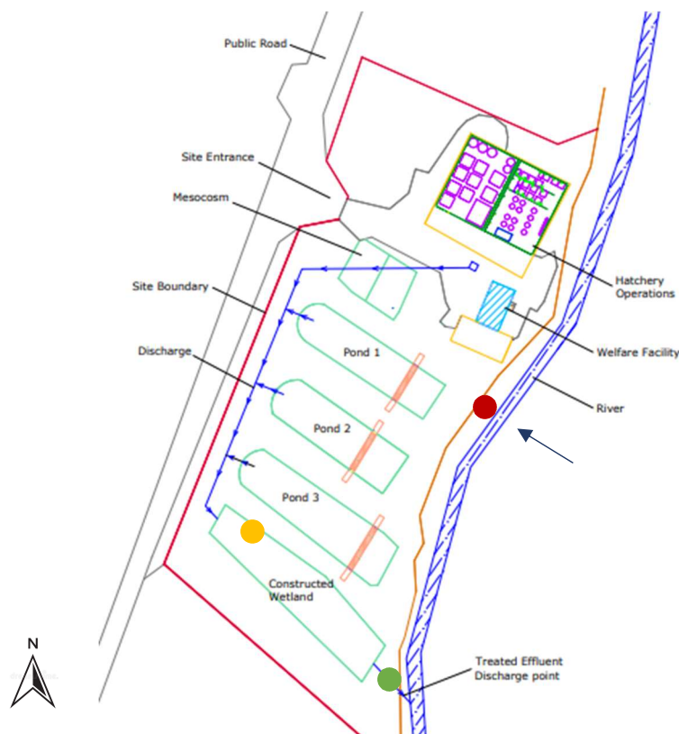
Figure 3.1: Schematic of Keywater Fish Farm. The location of the hatchery / nursery, mesocosms, culture ponds, settlement pond, which is included in the constructed wetland, and the holding tank at the discharge point are included. Blue lines indicate the direction of the flow of water. The red circle indicates the location of the intake sampling point . The green circle indicates the location of the output sampling point . The yellow circle indicates the location of the settlement sampling point . (Source: Morefish & EcoAqua Project)
