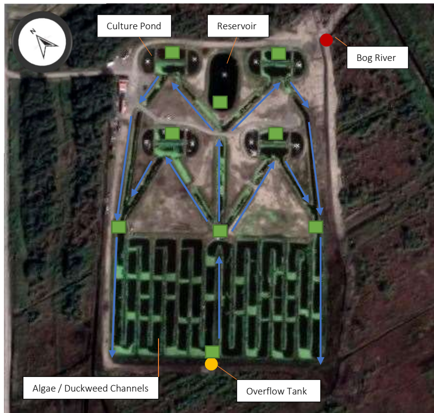
Figure 4.1: Aerial view of Oasis Fish Farm, located in Ballycon, Co. Offaly. The culture ponds, water reservoir, algae & duckweed wastewater treatment channels, overflow tank and bog river are all visible. Blue lines indicate the direction of the flow of water. The red circle indicates the location of the intake sampling point. The yellow circle indicates the location of the output sampling point. The green squares indicate all sampling points within the farm to monitor the IMTA process.
