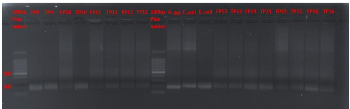
Figure 3.35 Agarose gel of DGGE 'nested' PCR samples 9-16 from FP & TP, A. salmonicida (abbr. A. sal) & E. coli .
