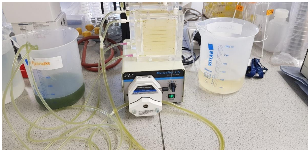
Figure 3.6 Vivaflow 200 system set up, with colour intensification of the sample during concentration.
