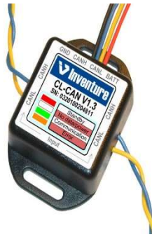
Figure 38: CAN-Clip sensing information on CAN-High and CAN-Low wires
