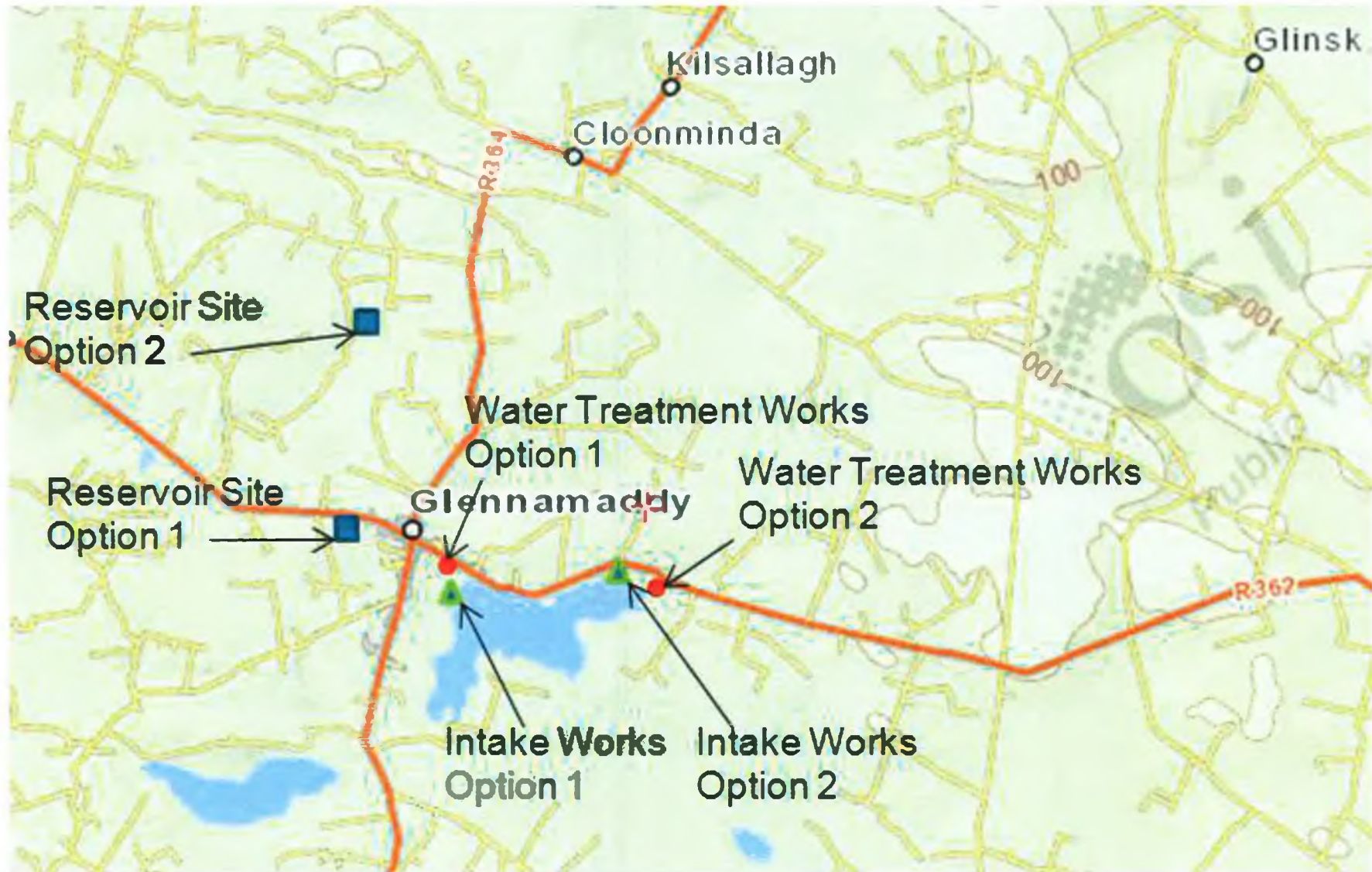
Map of Alternative sites for Reservoir, Intake Works and Water Treatment Works.
