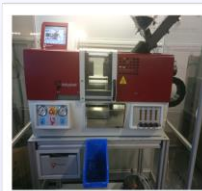
The Micro-injection molding machine is Babyplast 6/12 (Rambaldi, Italy).
