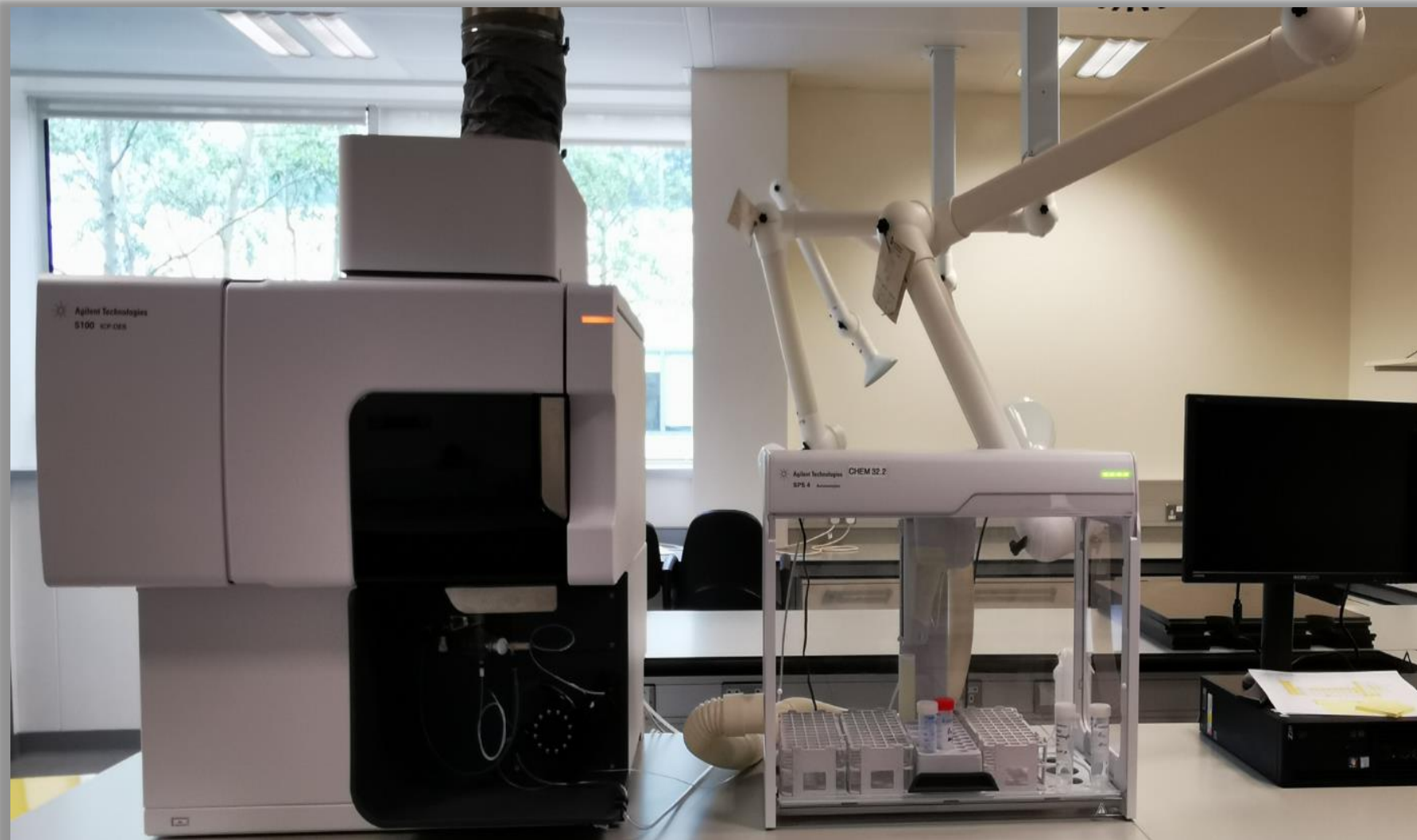
Vertical Dual View Optical Emission Spectrometer coupled with SPS4 Auto-sampling Unit
