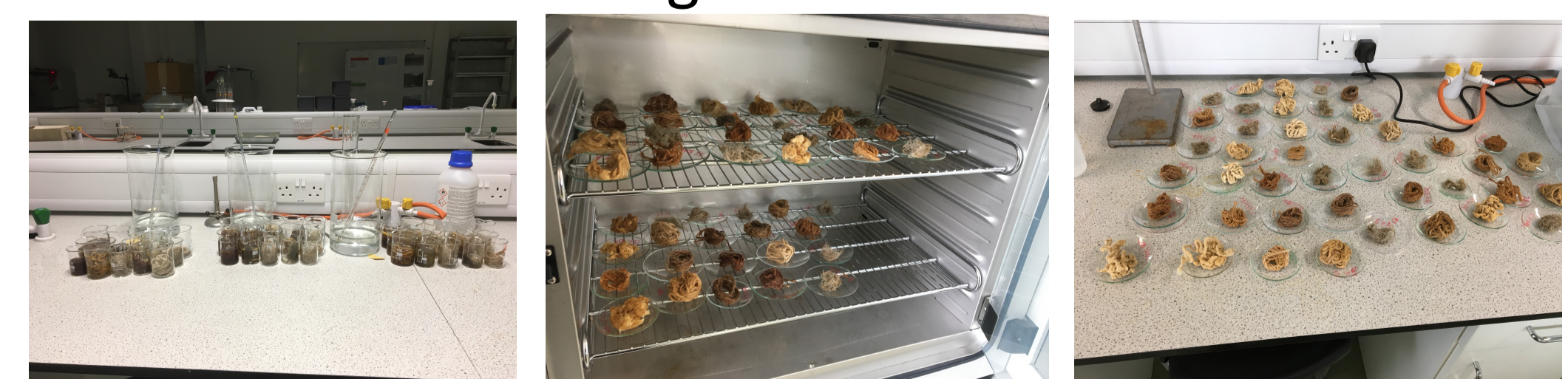
Figure 5: Samples of Jute, Hemp and Flax fibres during treatment (Left), drying (Centre), ready for tests (Right).
