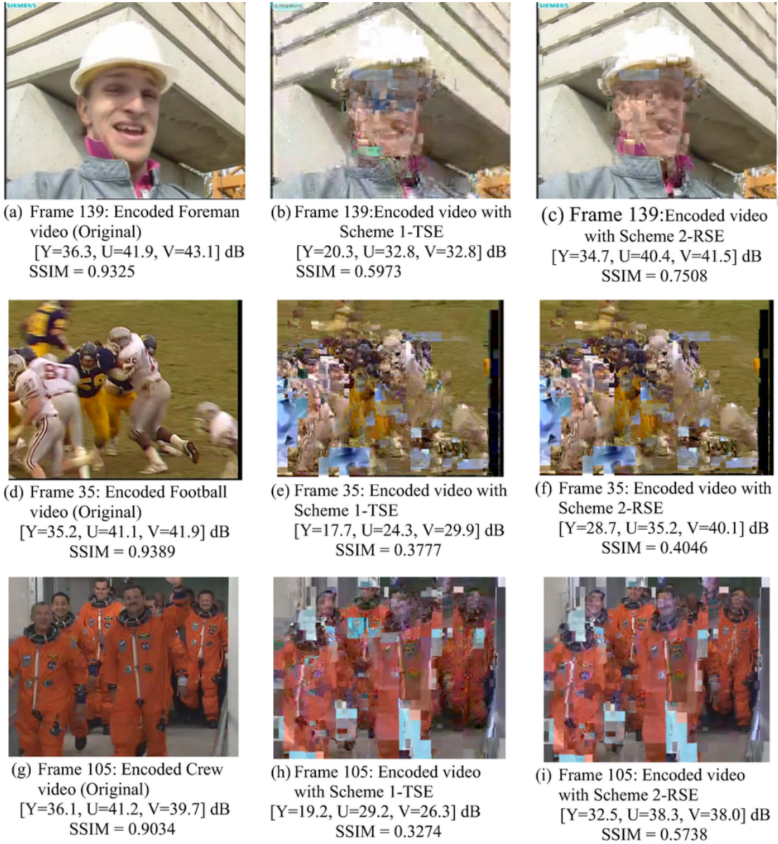
Fig. 13. Comparison of video frames encrypted with Scheme 1-TSE and alternatively with Scheme 2-RSE.
