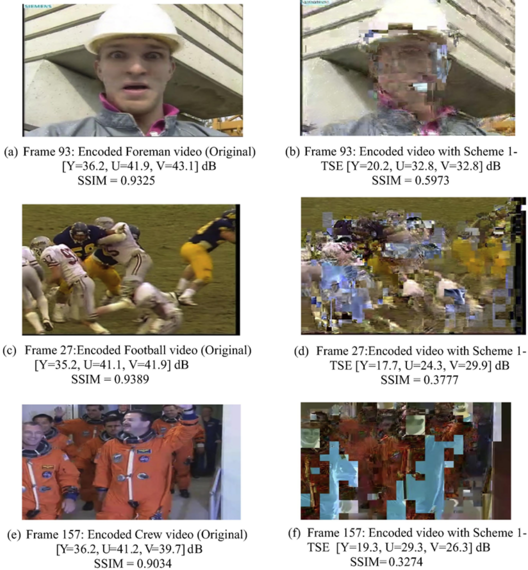
Fig. 5. Impact on video distortion and structural distortion of Scheme 1 SE at QP = 28.
