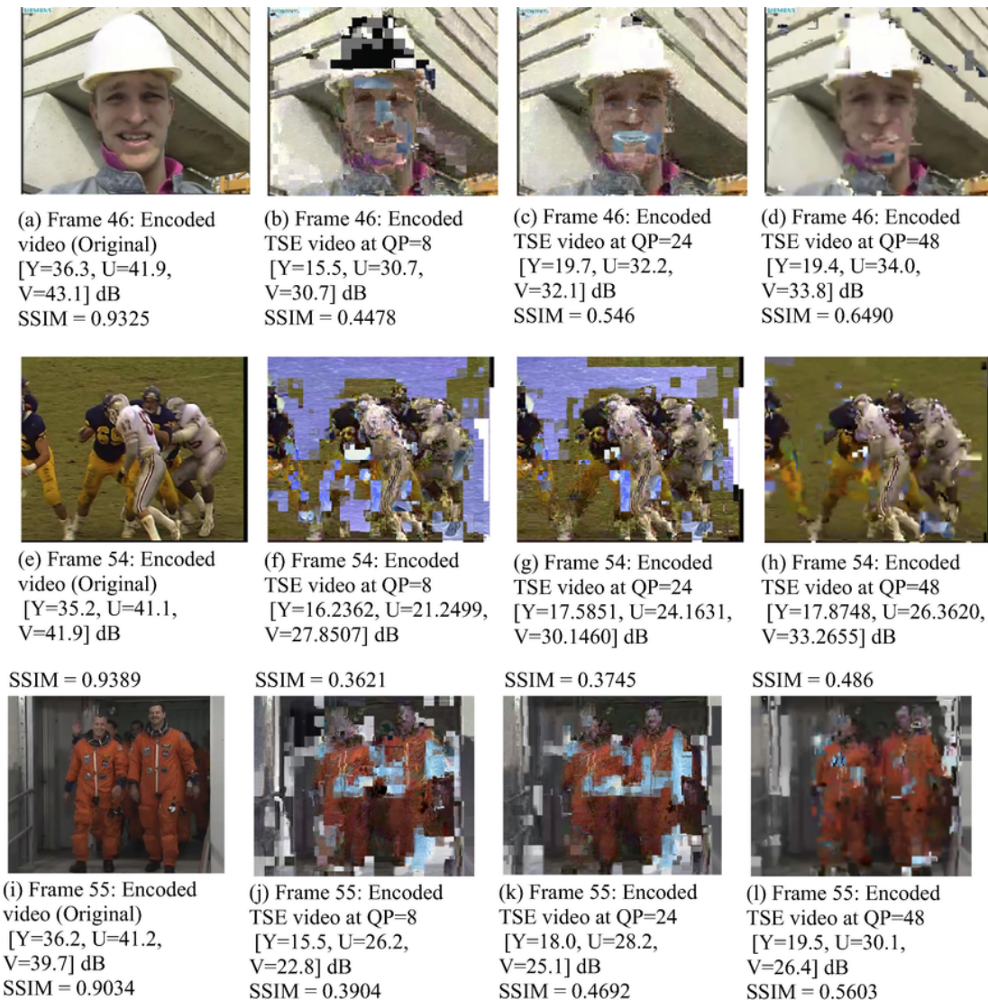
Fig. 7. Impact on video distortion and structural distortion of Scheme 1 i.e. SE with transparency.
