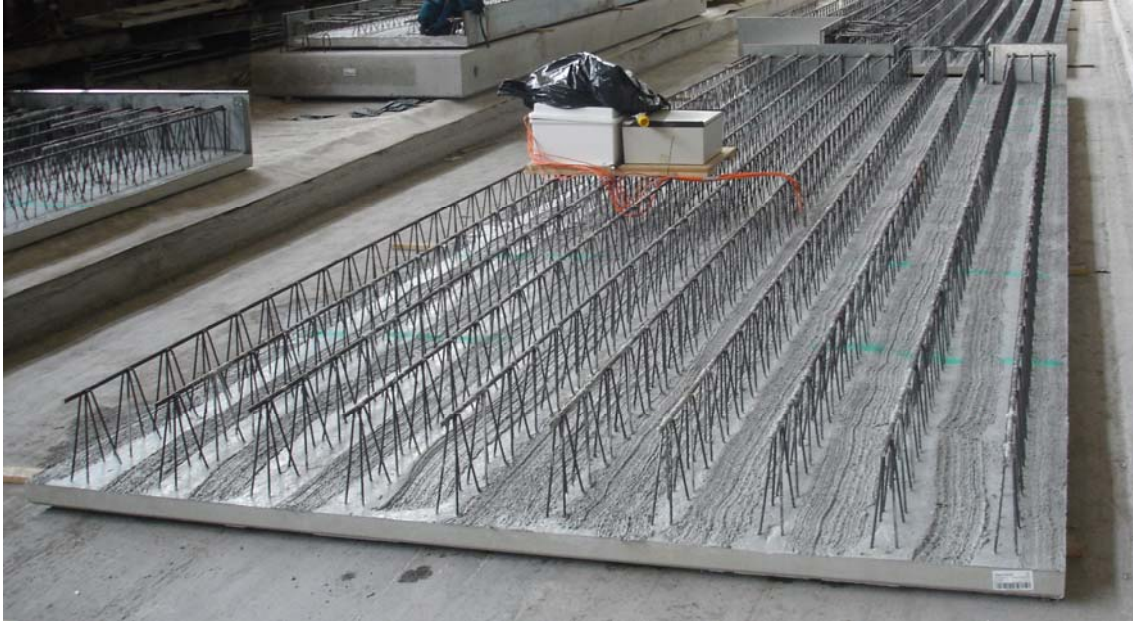
Figure 2. Precast Concrete Lattice Girder Plank (with embedded sensors)
