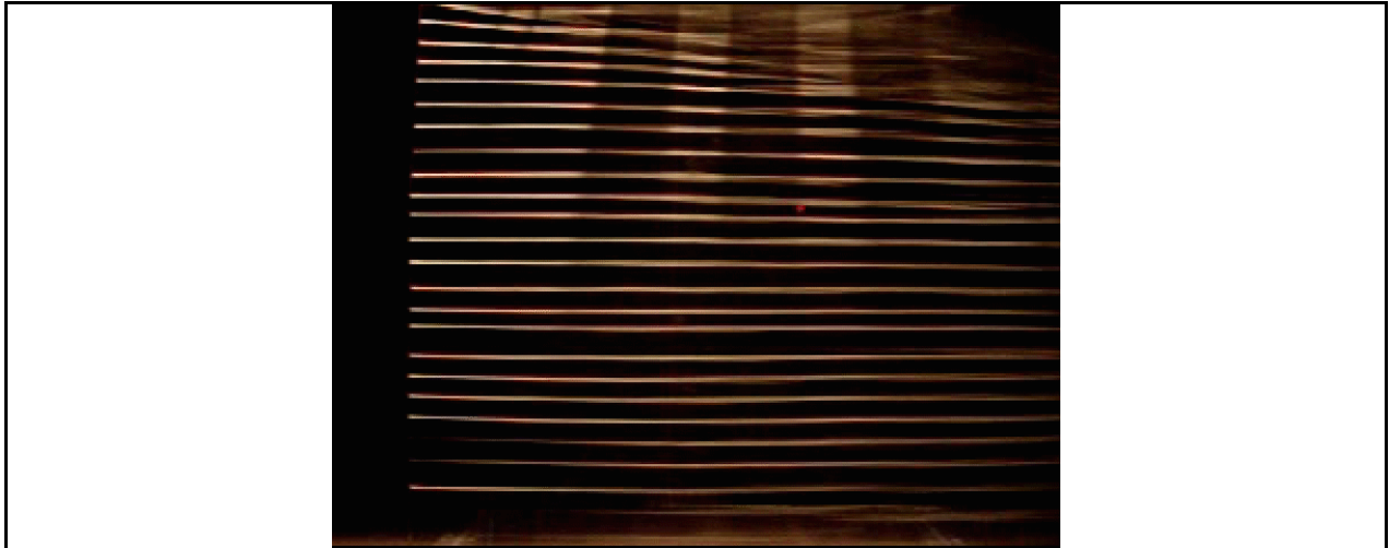
Figure 2 – Smoke streamlines recorded within the test section at a free stream velocity of 2m/s. Approximately 8 mm between each streamline.
