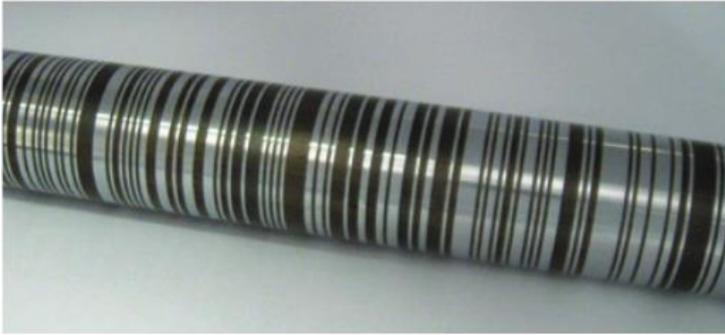
Figure 27 Marking applied on rod
