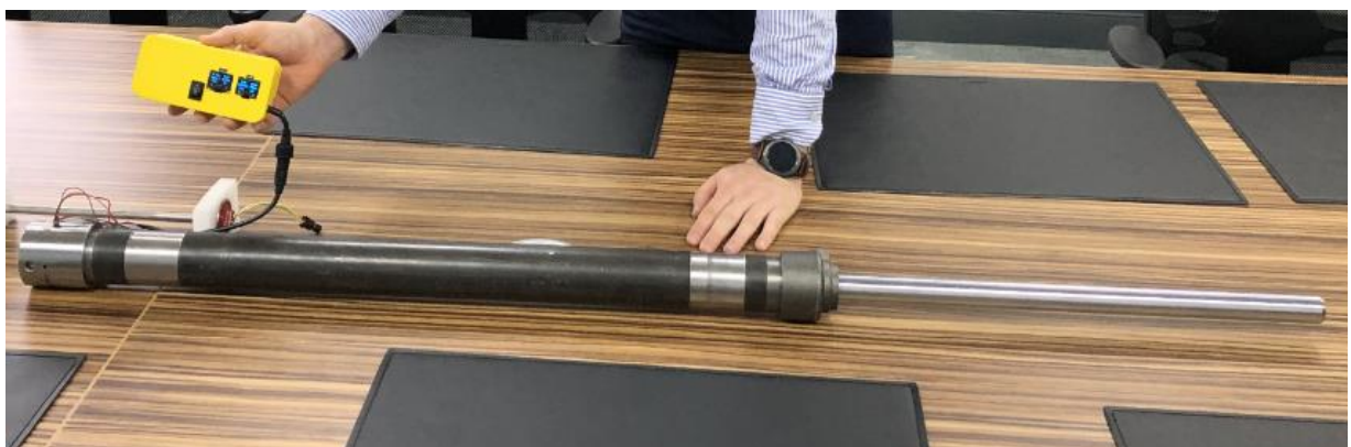
Figure 121 Sensor and dry operating cylinder assembly complete
