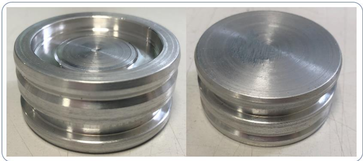
Figure 86 Turned aluminium body
