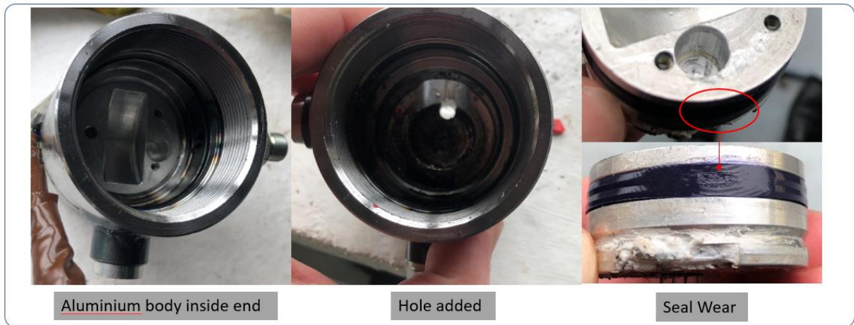
Figure 144 Dismantling of sensor
