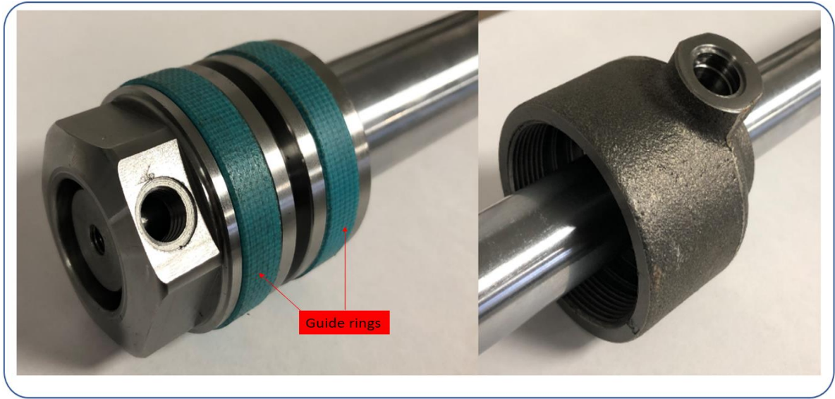
Figure 118 Assembling Gland and Piston
