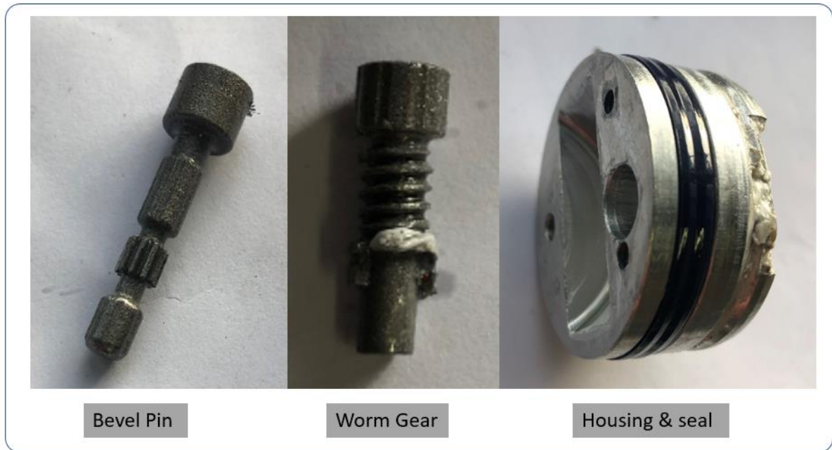
Figure 154 Examination of wearing parts
