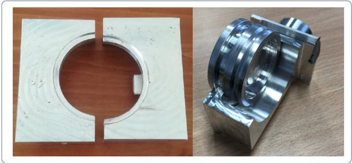
Figure 87 Fixture to secure turned part
