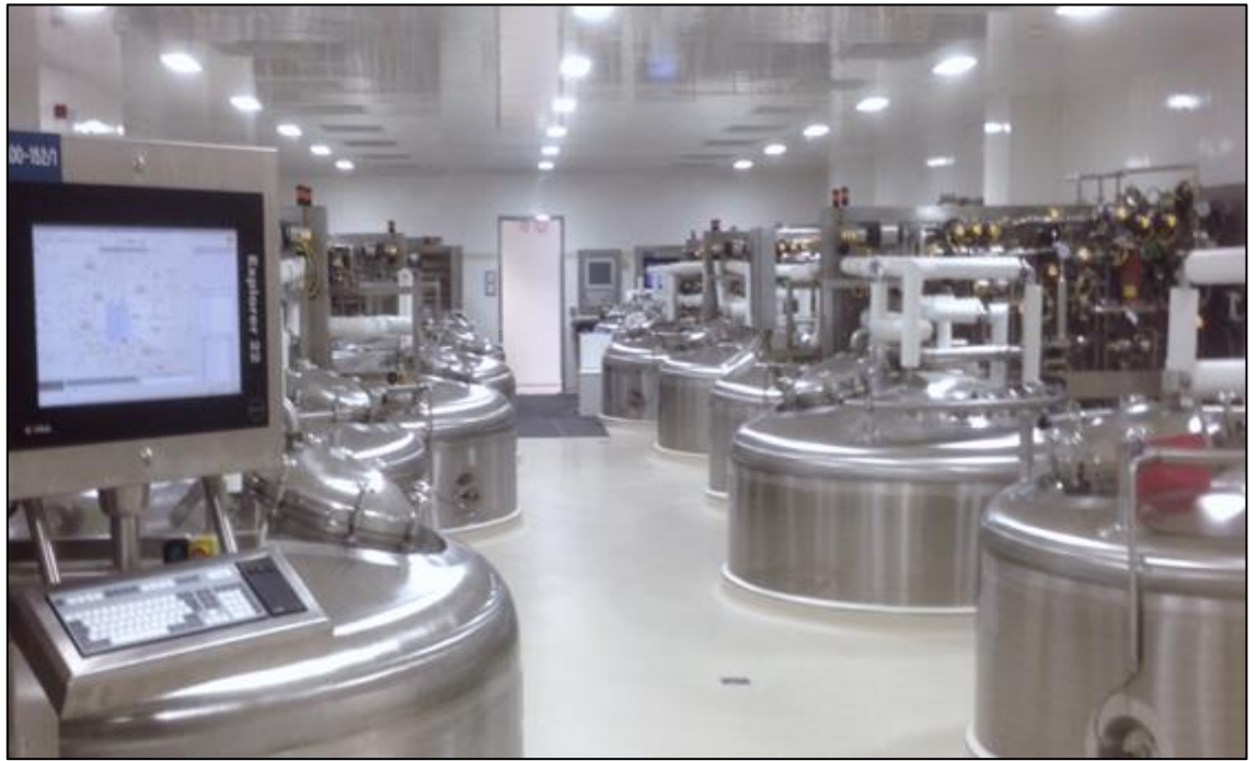
Figure 25 Conventional Buffer Preparation & Hold Systems
