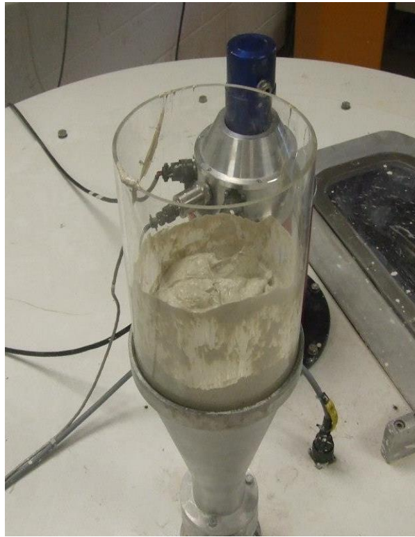
Figure 3.9: Fibrous sample fed into the funnel and descending onto the dispersion blades.
