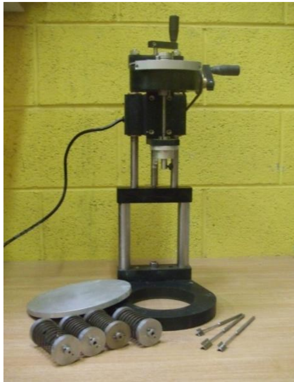
Figure 3.16: Electric Laboratory Vane Apparatus SL800, with accompanying blade and spring attachments.
