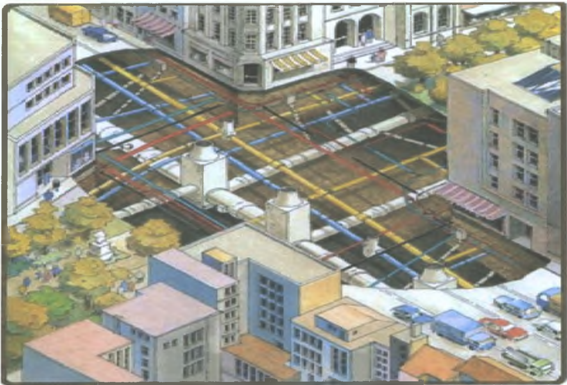
Fig 4.1 Typical underground infrastructure in an urban area
