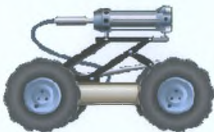
Fig 5.1 CCTV camera mounted on a tractor
