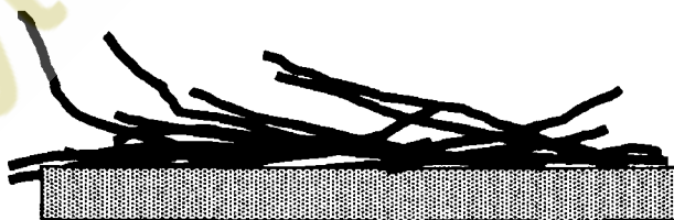
Figure 1.34. Immobilisation of DNA probe to gold electrode through adsorption.
