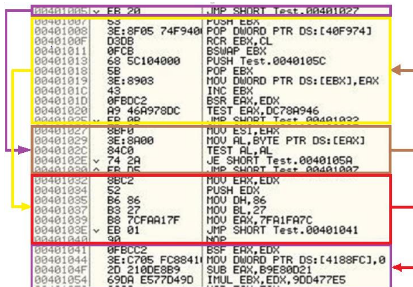
Figure 6: Code Transposition: transposition based on Unconditional Branches
